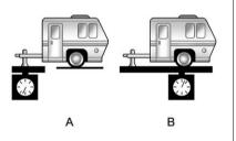
Using a weight-carrying hitch, the trailer tongue (A) should weigh 10 to 15 percent of the total loaded trailer weight (B).
